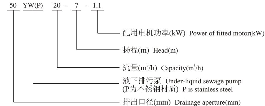
YW(P)系列液下排污泵结构示意图 Table of YW(P) series under-liquid sewage pump's structure drawing
