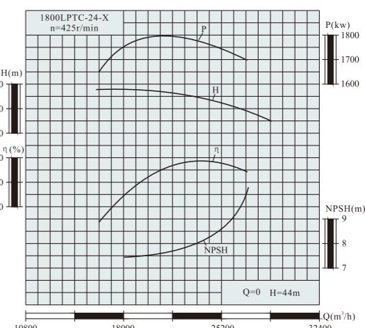
**LP(T)型性能曲线图 LP(T) type pump performance curve drawing**
