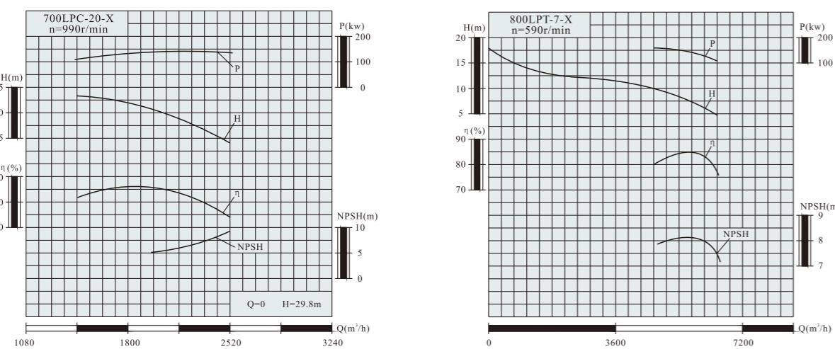
**LP(T)型性能曲线图 LP(T) type pump performance curve drawing**
