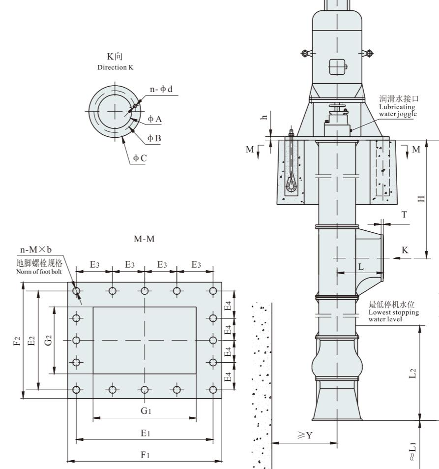
安装尺寸表(出口直径700mm以上、泵吐出口在基础之下) Installation Dimension Table (outlet diameter less than 700mm and outlet under the base)
