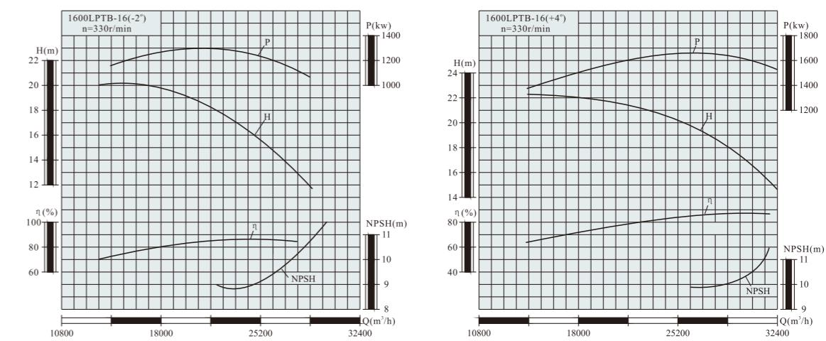
**LP(T)型性能曲线图 LP(T) type pump performance curve drawing**
