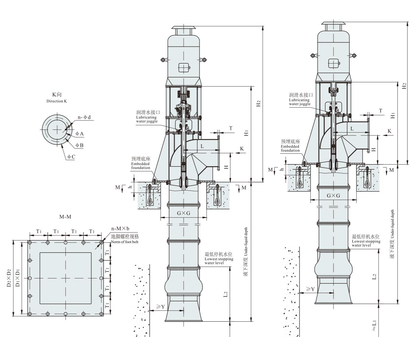
**LPTC抽芯式安装尺寸表 LPTC loose core type installation dimension table**
