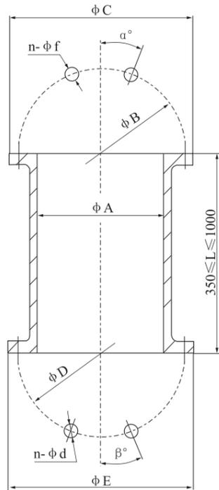
预埋管联接尺寸表 Connection Dimension Table For Pre-buried Pipe
