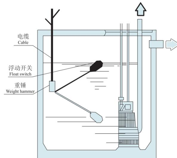
泵房布置简图 Pump station arrangement
